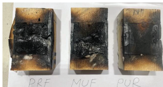
Figure 10 Specimens after fire test of bond line.
