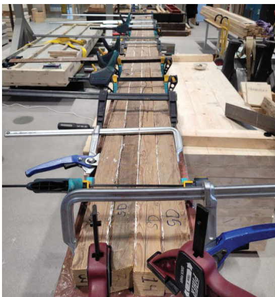
Figure 4 Assembly of freshly bonded glulam beam, secured with lace screws.
