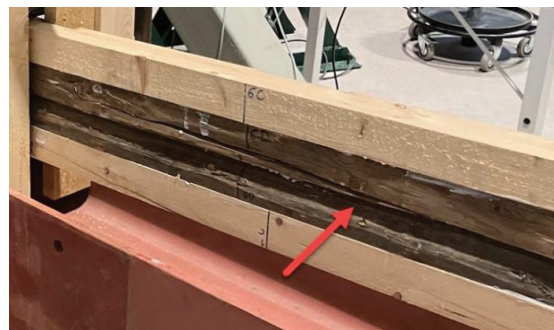
Figure 8 Insufficient contact surface between the lamellae.
