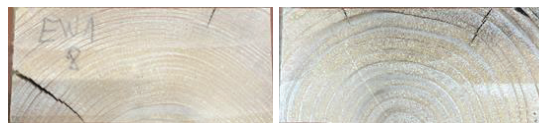
Figure 7. EW120 test specimens: Left – Timber sample with a charring result indicated by a red asterisk in Figure 8; right – Timber specimen of the remaining two samples from the same specimen ID.
