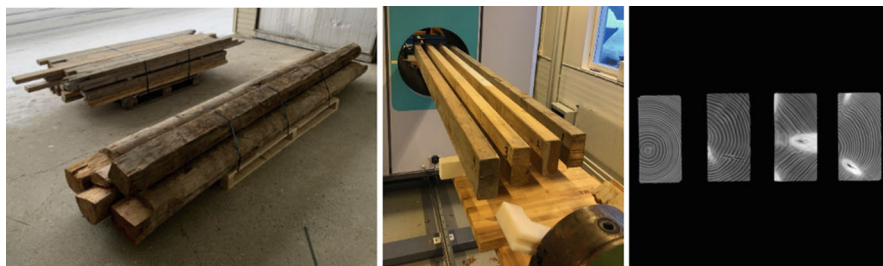
Fig. 2 56 planks and 5 barn timber logs (left), sample setup during CT scanning (middle) and a section of the scan (right)
